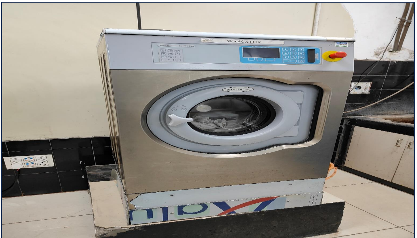
Washcator to test spirality and dimensional stability of fabric
