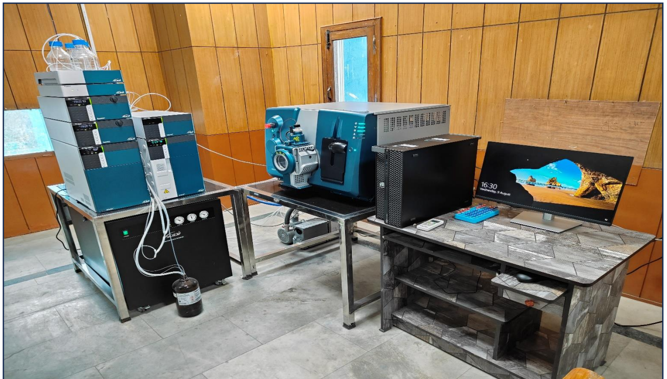
Liquid Chromatography Mass Spectrometer to test presence of Hazardous components in Leather, Textiles, PVC, Polymer
