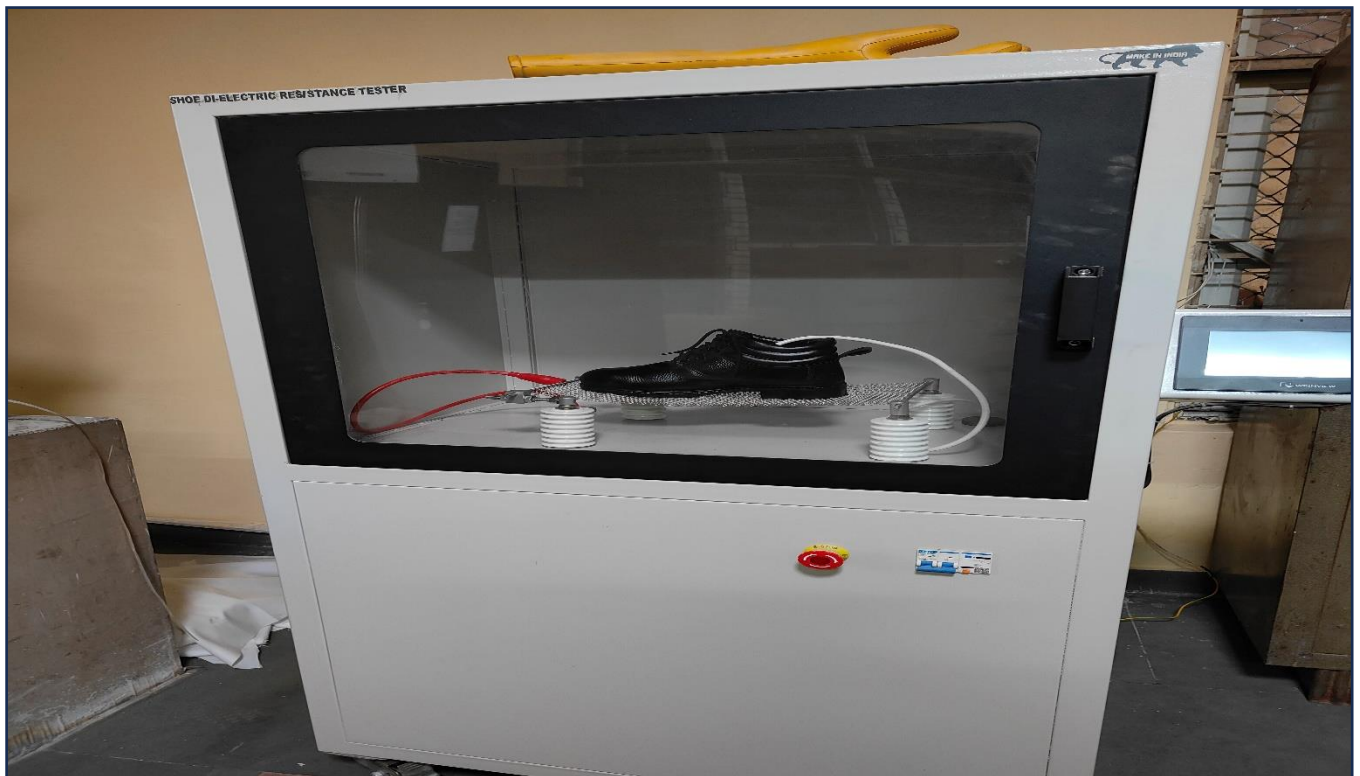
High Voltage Tester to check shoe performance of high voltage withstand and current leakage
