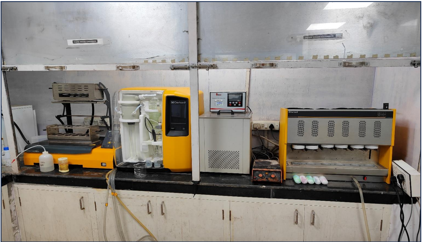
Soxhlet Apparatus with nitrogen analyzer to test sample extraction and fat content
