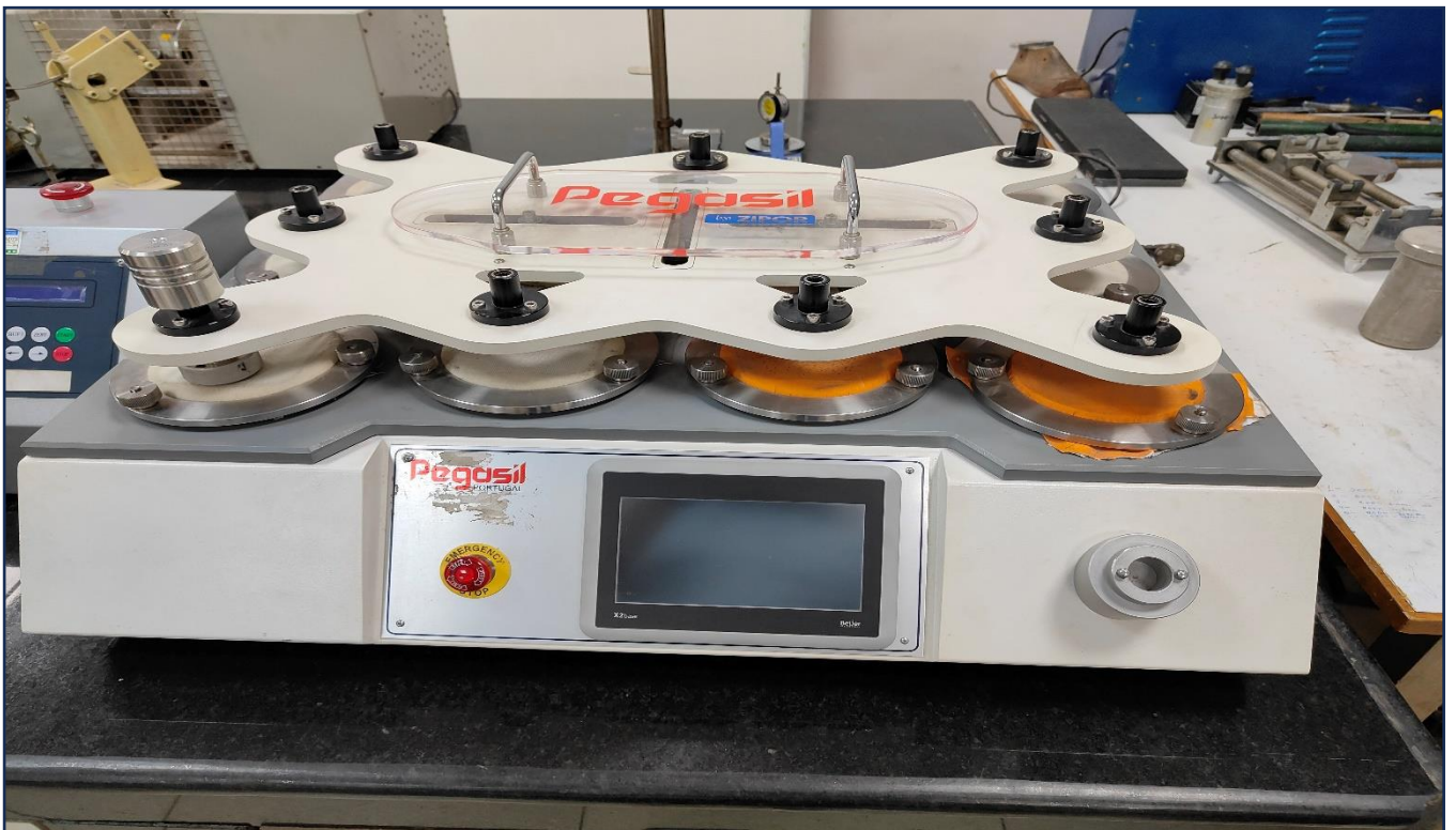
Abrasion Tester (Martindale) to check the resistance of a material to wet and dry abrasion
